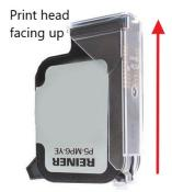
1) The yellow ink cartridge must be stored in "nozzle up" position to keep the nozzles in good condition. Make sure cartridge is stored with the plastic clip on as shown in picture, as well as info in foil pouch the cartridge comes in.
